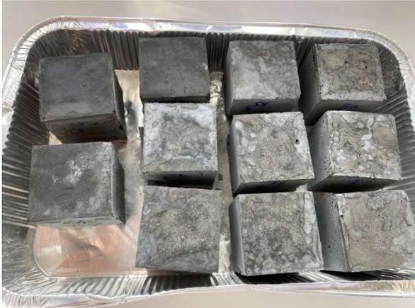
Specimens of geopolymers with different SS:HS ratios
