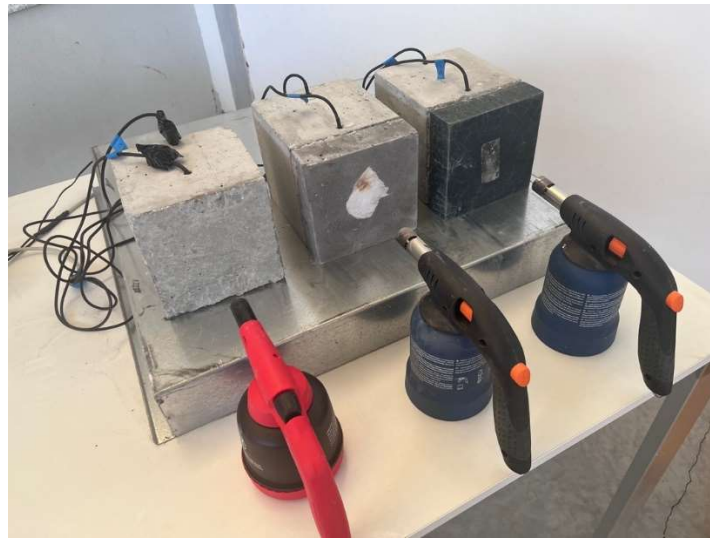
Fire Testing setup illustrating the placement of thermocouples for monitoring temperature fluctuations inside specimens.
