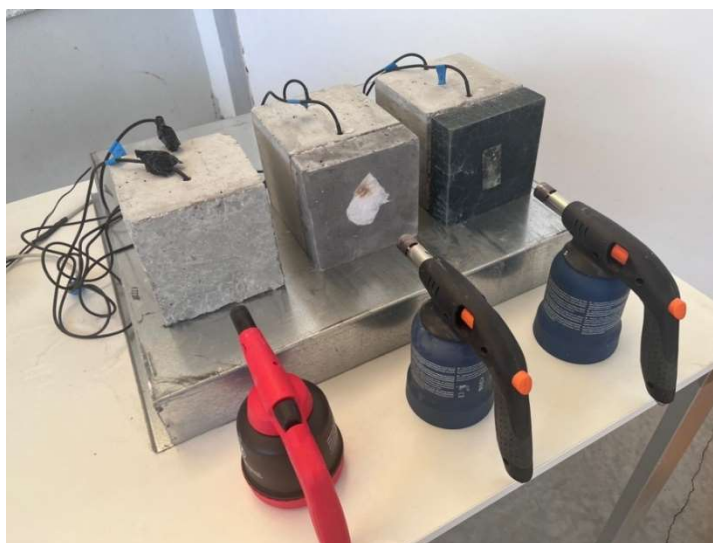
Figure 14: Fire testing setup illustrating the placement of six thermocouples for monitoring temperature fluctuations inside concrete cubes.
