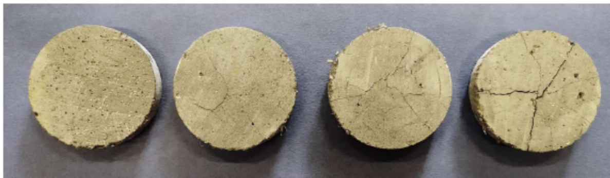
Figure 1. Under-surface of specimens after impact from heights of 0.5m, 1.0m, 1.5m and 2m (left to right). Appreciable deformation and multiple cracking is observed. Energy dissipation is evident by crack bridging and by the steel fibers.
