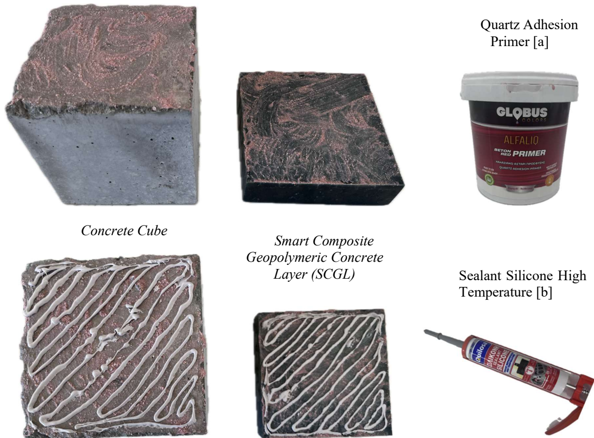
Figure 12: Application of quartz adhesion primer [a] and sealant silicone [b] on the Surfaces of smart composite geopolymeric concrete and concrete cube.
