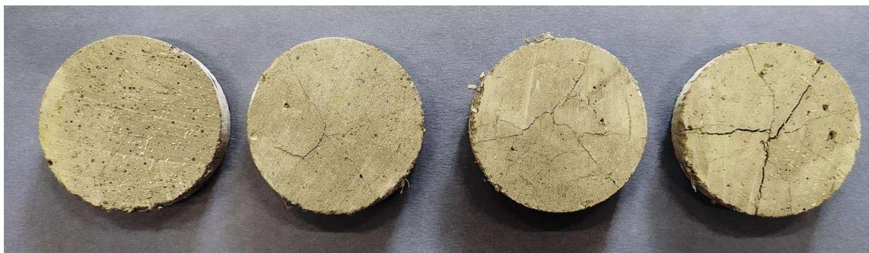
Figure 19: Under-surface of specimens after impact from heights of 0.5m, 1.0m, 1.5m and 2m (left to right).
