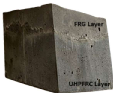
Figure 1: Hybrid Laminated Materials (HML) layers, on top the FRG Layer and at the bottom the UHPFRC Layer.
